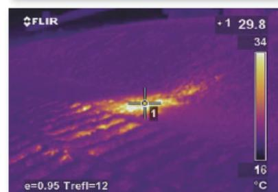
Heating, self-combustion monitoring in power station coal stock
